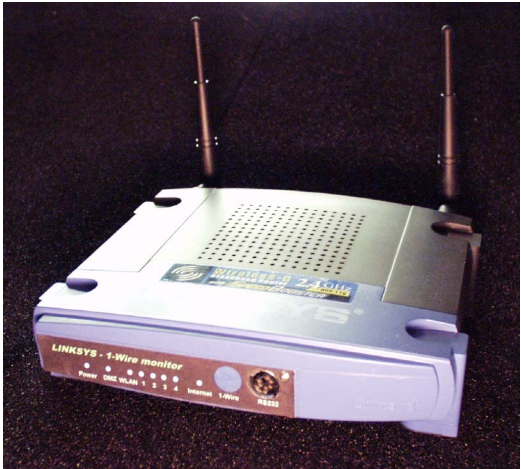
Figure 6 – Image of another LINKSYS WRT54GS unit, this time with only the addition of the RS232-F port. The 1-Wire was not brought out on the case since the internal 1-Wire functions were all that were needed for this particular unit.
