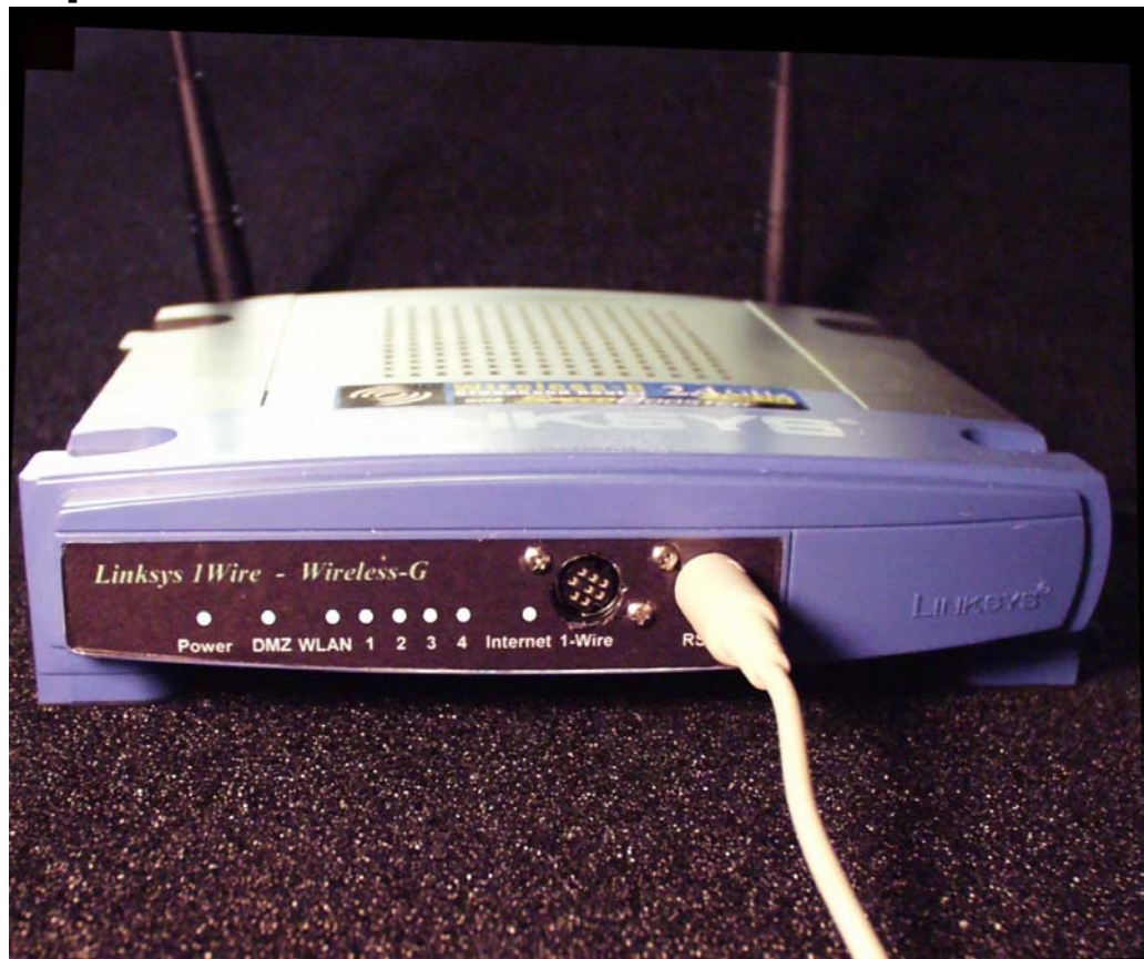
Figure 4 – LINKSYS WRT54GS modified with LP-LINKSY-1W installed. Note the new front label and the added Mini-Din jacks for 1-Wire and RS232 on the front of the unit. We have designed the case modifications to be as easy and simple as possible.
